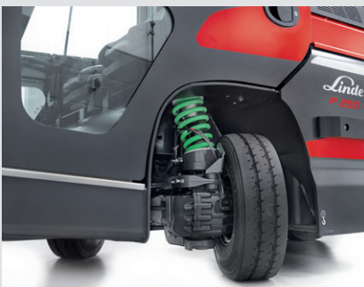
Coil spring and maintenance free braking system
